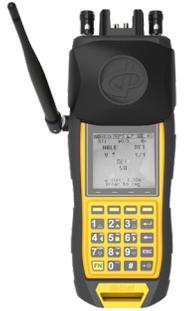
Therefore, normal GPS accuracy is not suitable for blast hole positioning. This is why Detnet has developed a user-friendly Differential-GPS (DGPS) system which is fully integrated with the CE4 Tagger and Commander system. The system provides sub one-meter accuracy for accurate blast hole tagging/logging.
